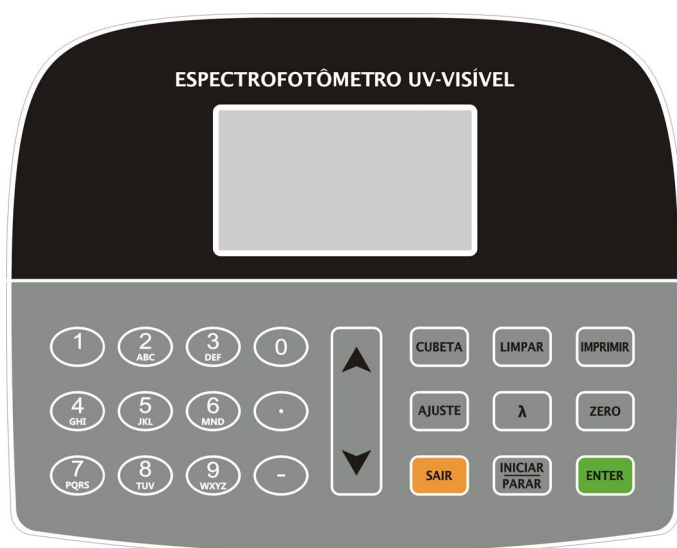
Fig 2-2 Painel de Controle
